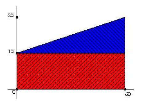
If the total distance travelled is represented in this example, as in the case of constant speed, by the area under the speed graph between t=0 and t=60, then it is  $60 \times 10 + \frac{1}{2}(60 \times 10) = 900$  metres.
