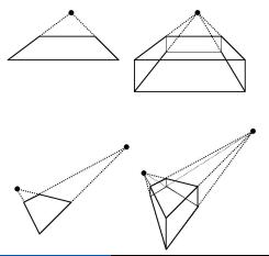
One-point and two-point perspective drawings of a rectangle and retangular box.
